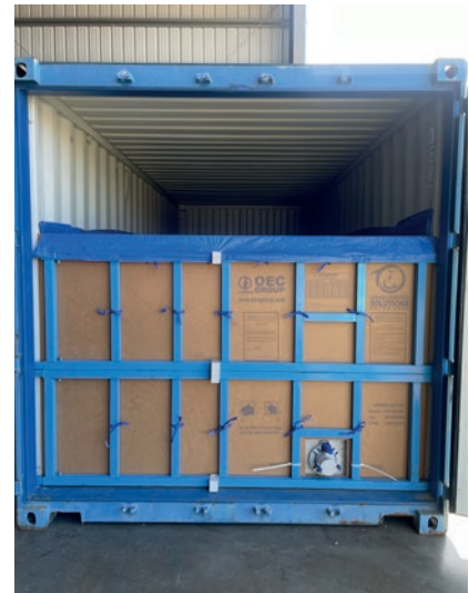
Picture 6 - An example fitted bulkhead (Image Courtesy of OEC Group)
